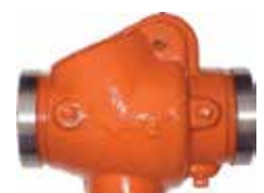
NCI Swing Check Valve CKVA-GD8351 350 PSI, D.I. Body, Rubber Disc, Bronze Seat. • Size: 2"-8" Grooved
