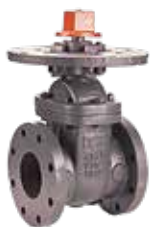
NIBCO Gate Valve F609/M609 175 PSI, C.I. Body, N.R.S., Solid Wedge, Indicator Post Pattern. • Size: 4"-12" FLG or Mechanical
