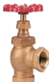
NIBCO Bronze Angle Valve KT-67-UL 175 PSI, Screwed Over Bonnet, Rubber Disc. • Size: 1/2"–1" Threaded
