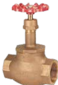
NIBCO Bronze Globe Valve KT-211-W-UL 175 PSI, Screwed Over Bonnet, Rubber Disc. • Size: 1 1/4"–3" Threaded
