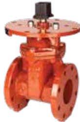
NIBCO Gate Valve F-609-RW 300 PSI, Lead Free, D.I. Body, Resilient Wedge, Indicator Post Pattern. • Size: 4"-12" FLG x FLG • AWWA509/515, NSF/ANSI 372
