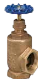
NIBCO Bronze Angle Valve T-301-W 175 PSI, Screwed Over Bonnet, Rubber Disc. • Size: 1 1/4"–3" Threaded
