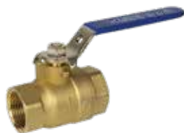
NCI 2-Piece Brass Ball Valve (T/S)FP600 150 SWP • 600 CWP Size: 1/4"–2" • 400 CWP Size: 2 1/2"–4" • Threaded or Solder
