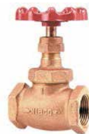
NIBCO Bronze Globe Valve KT-65-UL 175 PSI, Screwed Over Bonnet, Rubber Disc. • Size: 1/4"–1" Threaded
