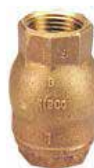
NIBCO Bronze Lift Check Valve T-480 250 PSI, Spring Actuated In-Line Lift, Buna-N Disc, Integral Seat. • Sizes 1/2"–2" Threaded
