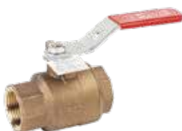
NIBCO 2-Piece Bronze Ball Valve KT-585-70-UL / KT-580-70-UL • 300 PSI Full Port, 1/4"–1" • 300 PSI Standard Port, 1/4"–2" • Threaded
