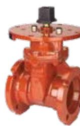
NIBCO Gate Valve M-609-RW 300 PSI, Lead Free, D.I. Body, Resilient Wedge, Indicator Post Pattern. • Size: 4"-12" FLG x Mechanical • AWWA509/515, NSF/ANSI 372
