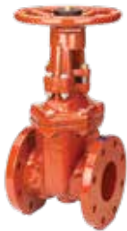
NIBCO Gate Valve F-607-RWS 300 PSI, Lead Free, D.I. Body, OS & Y, Bolted Bonnet, Solid Resilient Wedge. • Size: 2½"-12" FLG x FLG • AWWA509/515, NSF/ANSI 372
