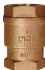
NCI Bronze Lift Check Valve CKVB-TBZ2373 300 PSI, Spring Actuated In-Line Lift, NBR Disc Ring, Integral Seat. • Sizes 1/2"–2" Threaded
