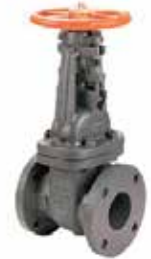
NIBCO Gate Valve F607-OTS 175 PSI, C.I. Body, OS & Y, Solid Wedge. • Size: 2½"-12" FLG x FLG
