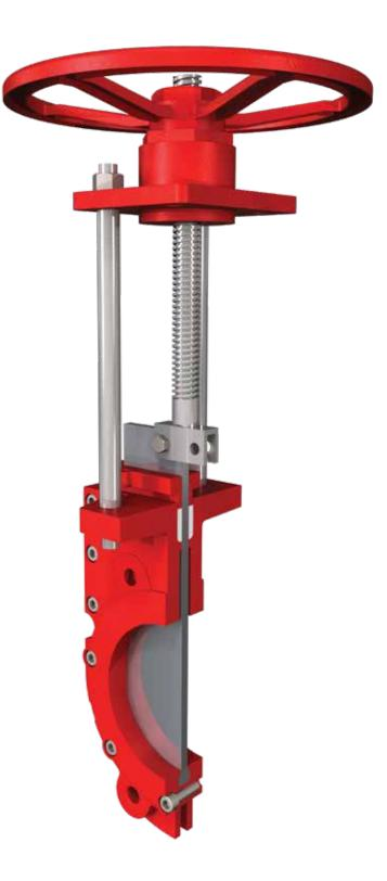
The Flow+ K2500 General Purpose Knife Gate Valve brings both performance and value to the table. This valve comes standard in either 304SS or 316SS with metal or Viton seats. The design complies with AWWA C520, TAPPI-TIS 405, and MSS-SP81 standards.
